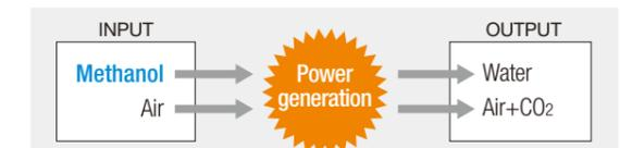
DMFCs generate electricity by producing a chemical reaction using methanol and air. DMFCs can continuously supply electricity as long as they are filled with methanol.
