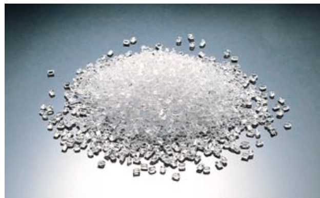
IUPILON polycarbonate resin pellets have applications ranging from electronic and office equipment to automobiles.
